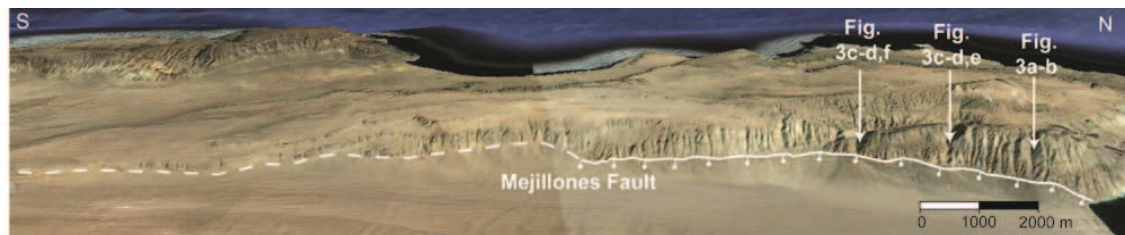
Figure 4. Oblique view of the Mejillones Fault scarp on Google Earth. White vertical lines depict the deepest and largest valleys, which cut across the western flank of the Mejillones Horst. The presence of S2 is restricted to the areas where these valleys drain. The white continuous line corresponds to the portion of the fault where the scarp is developed. The white segmented line indicates the fault segment where no scarp was present.
