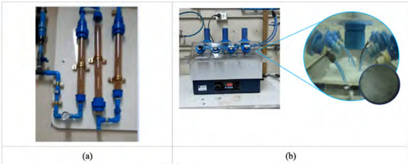
Figure 3. Main components of the laboratory-scale prototype: (a) acrylic adsorption columns packed with silica gel, and (b) assisted brine evaporation tank with hermetic sealing, temperature control, and porous-tip lances for dry-air injection.
