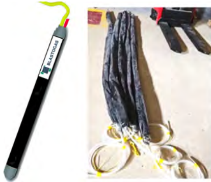
Figure 3. Representation of a BlastoGas cartridge (left); and empty cartridges ready for transportation (Oxquímica, 2024).
