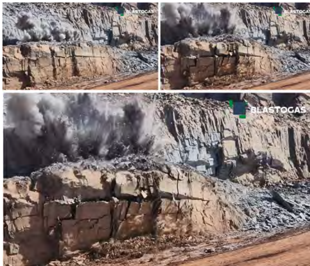
Figure 6. Phases of a BlastoGas LOX shot. Being an expansion of gases, one clearly notices the progressive opening of the natural joint present on the bench face (Oxquímica, 2024).
