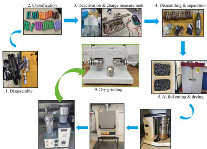
Figure 1. Pretreatment flowchart for the Spent LIBs
